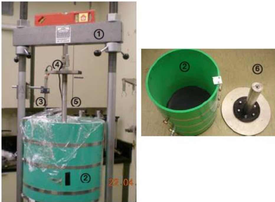
Fig. 1. Test setup for model pile loading test: ① Adjustable height loading frame ② Test tank ③ LVDT ④ Load cell ⑤ Model pile, ⑥ Compaction base plate.
