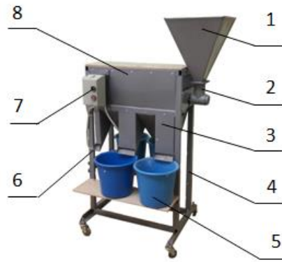
Fig. 5. Cylinder separator: 1 – hopper; 2 – feeder; 3 – discharge tray; 4 – frame; 5 – tank for the products of screening; 6 – separator drive; 7 – electric panel; 8 – housing of the separator
