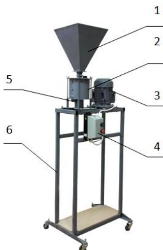
Fig. 2. Huller: 1 – grain hopper; 2 – the body of the huller; 3 – electric motor; 4 – control panel; 5 – outlet branch pipe; 6 – bench
