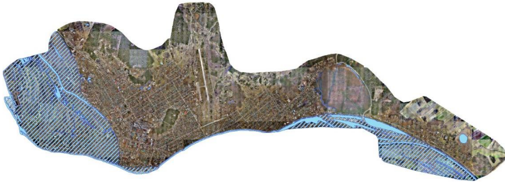
Fig. 4. Orthophotomap of Kolpashevo city with a flood zone at a water level +8 m
