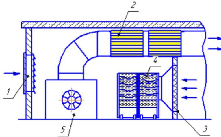
**Figure 1.** Scrubber placement scheme: 1 – shutter of fresh air supply, 2 – bactericidal device, 3 – valve for supply of polluted air from the poultry house, 4 – scrubber, 5 – air supply fan in the built in ducts of cage batteries.
