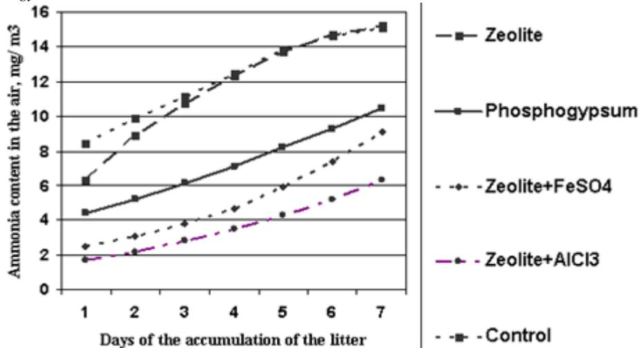
**Figure 2.** Dynamics of ammonia content in the air of the poultry house, depending on the substances used in the scrubber.
