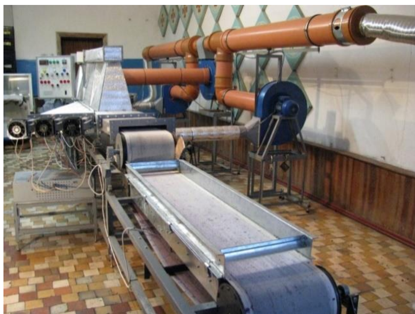
Fig. 1. Equipment for seed irradiation with MWF of EHF developed by Kharkiv National Technical University of Radio Electronics, installation of a microwave design of the "UMVK-1" brand
