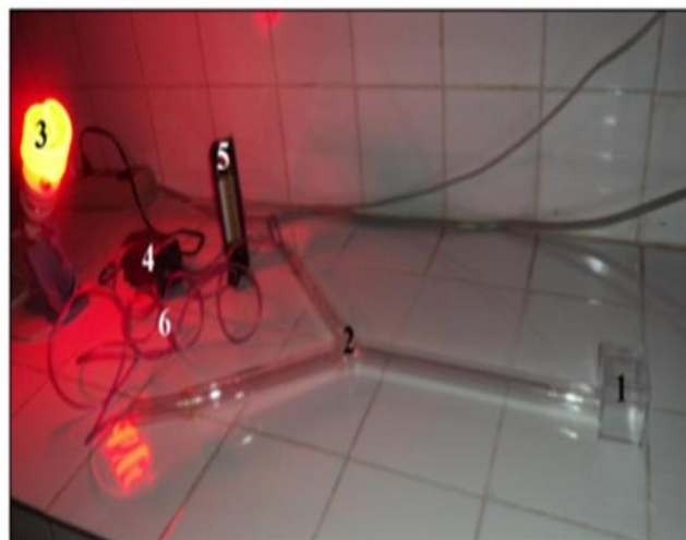
Fig. 1. Two-way Y. 1. Starter Box Olfactometer; 2. Olfactometer; 3. Red lamp; 4. Compressor; 5. Flow meter; 6. Air inlet pipes (Habbach, 2013).
